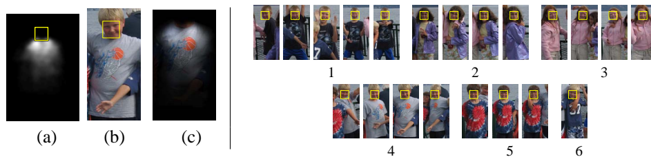
Figure 2: Left: (a) Spatially weighted mask shown relative to a face detection. Brightness indicates weight. This mask is used to weight contributions to a color histogram describing each person’s clothing. (b) Cut out of a person with face detection superimposed. (c) Weight mask superimposed over the image. Right: (1)-(6) The clusters correctly computed for the six different people found in the photos shown in figure 1.
