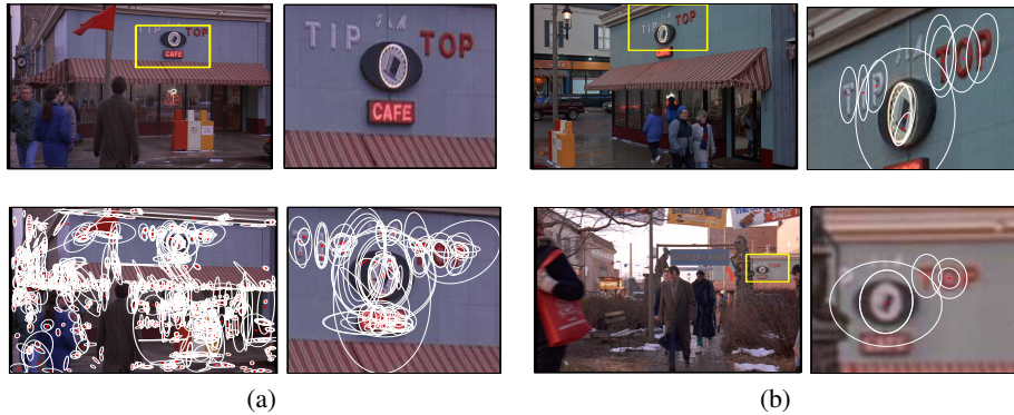
Fig. 1. Object query example I. (a) Top row: (left) a frame from the movie ‘Groundhog Day’ with a query region in yellow and (right) a close-up of the query region delineating the object of interest. Bottom row: (left) all 1039 detected affine co-variant regions superimposed and (right) close-up of the query region. (b) (left) two retrieved frames with detected region of interest in yellow and (right) a close-up of the images with affine co-variant regions superimposed. These regions match to a subset of the regions shown in (a). Note the significant change in foreshortening and scale between the query image of the object, and the object in the retrieved frames. Querying all the 5,640 keyframes of the entire movie took 0.36 seconds on a 2GHz Pentium.
