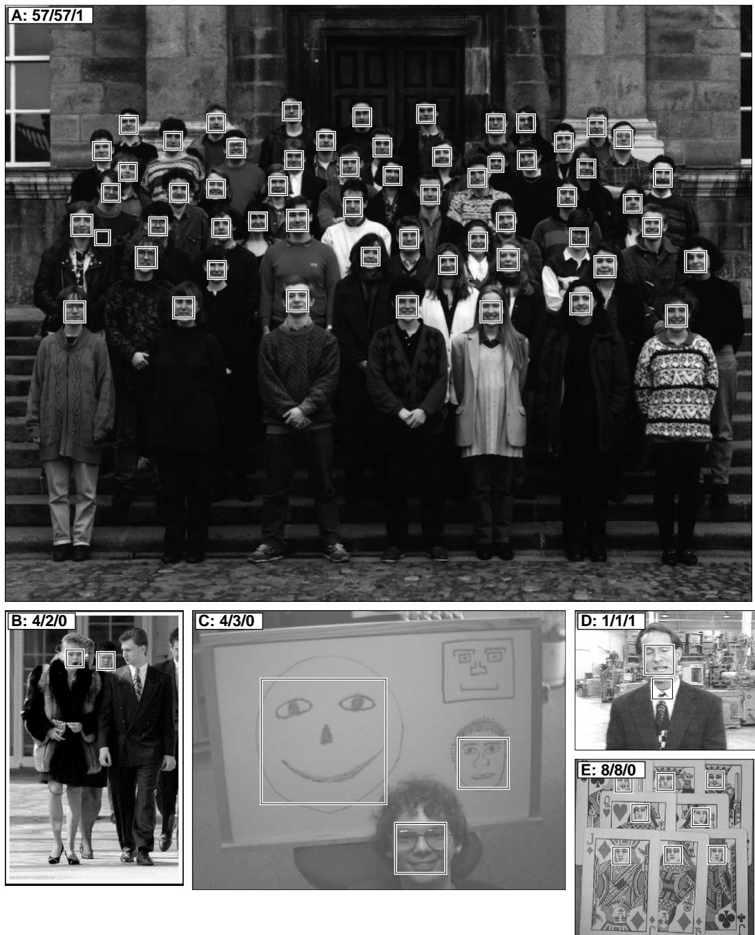
Figure 11: Output obtained from System 11 in Table 1 on images from Test Set 1. For each image, three numbers are shown: the number of faces in the image, the number of faces detected correctly, and the number of false detections. Some notes on specific images: Faces are missed in B (one due to occlusion, one due to large angle) and C (the stylized drawing was not detected at the same locations and scales by the two networks, and so is lost in the AND). False detections are present in A and D. Although the system was trained only on real faces, some hand drawn faces are detected in C and E. A was obtained from the World Wide Web, B and E were provided by Sung and Poggio at MIT, C is a CCD image, and D is a digitized television image.
