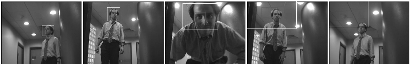
Figure 2. The sequence depicted in Figure 1 tracked with an adaptive colour model. Here, the model adapts to cope with the change in apparent colour.
