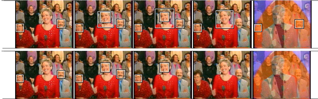
Fig. 4. Face detection improvement. Upper sequence represents the frame by frame face localization, whereas the bottom sequence is the improved face detection. We can note that faces are not detected in the dissolve, while the three main characters are all detected at least one time in the sequence.
