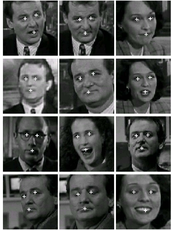
Figure 7. Automatically detected facial features: High accuracy is achieved in spite of wide variation in facial expression, pose, illumination and the presence of facial wear (glasses).
