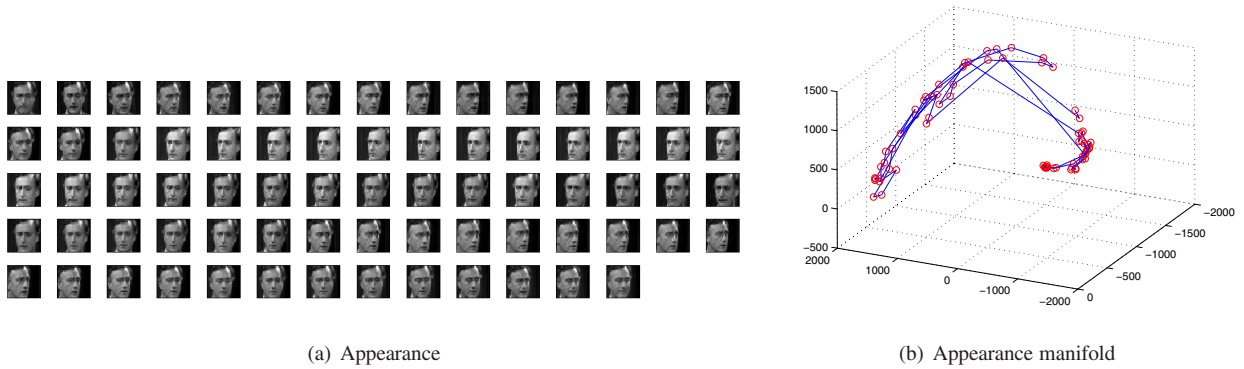
Figure 4. A typical face track obtained using our algorithm. Shown are (a) the original images are detected by the face detector (rescaled to the uniform scale of 50 \times 50 pixels) and (b) as points in the 3D principal component space with temporal connections.
